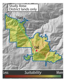
C. Slope, Aspect, & Creeks Scenario C's suitability surface included slope, aspect, and the creek buffers, and was constrained to lands owned by Midpen.
