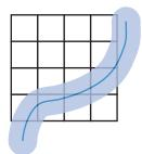
Overlay of creek centerline and 50-foot buffer on raster grid
