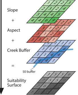
Figure 5.9. Preparing the suitability surface. The reclassified layers are combined into one grid with each cell's value representing the suitability for trail building. *Source*: Author.
