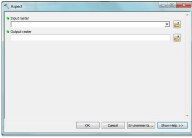
Input Raster:Digital Elevation ModelOutput Raster:Aspect Surface
