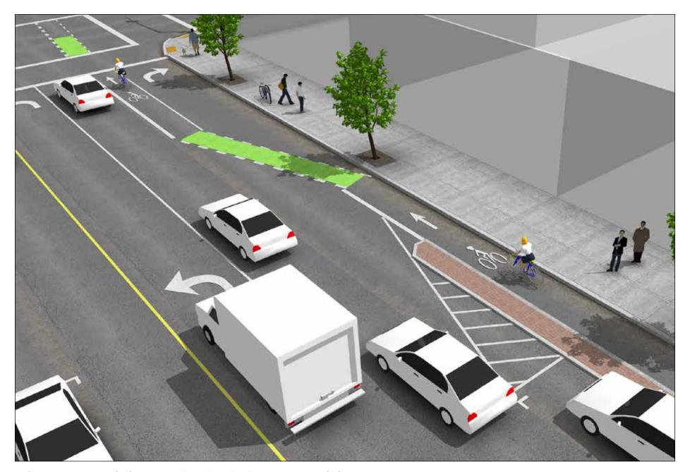
**Figure 3.23**: An Example Showing How Green Paint Can Connect Fragmented Bike Lanes. Source: Simes, Randy. 2012. Cincinnati becomes the first Ohio city to install green bike lanes. UrbanCincy. http://www.urbancincy.com/2012/11/cincinnati-becomes-second-ohio-city-to-install-green-bike-lanes/ (accessed November 19, 2012).
