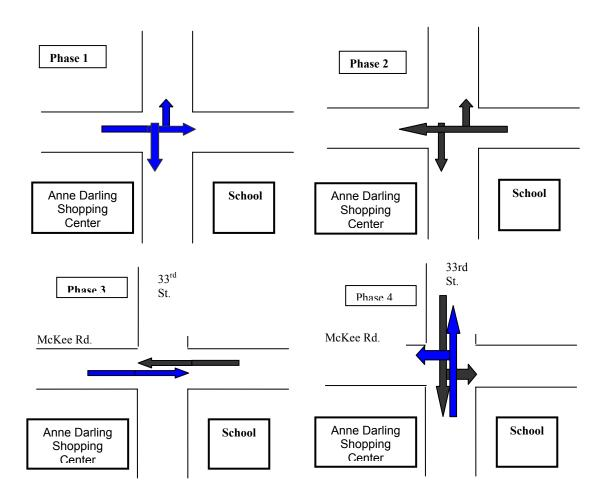
Figure 36 - Current Signal Phasing
