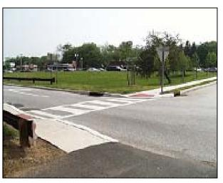
**Figure 31 -** Example of ladder crosswalk Source: http://tid1s0.engr.ccny.cuny.edu/utrc/CrosswalkSafety.pdf
