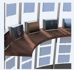
Top and bottom sheet metal is reclaimed local manufacture waste.
