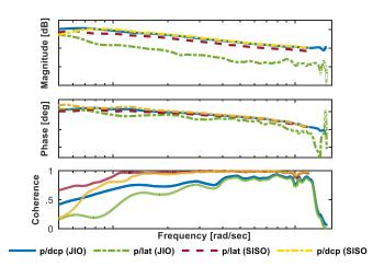
Figure 9. DCP and Lateral Cyclic to roll rate frequency response.
