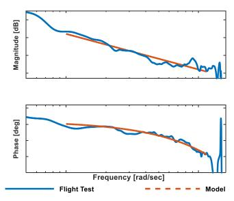
Figure 13. Lateral Cyclic to roll rate frequency response from JIO and low order transfer function approximation.
