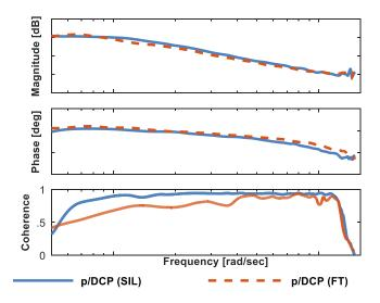
Figure 10. Flight Test and SIL comparison of DCP to roll rate frequency response.
