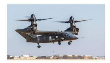
Figure 1. V-280 in VTOL Mode flight.
