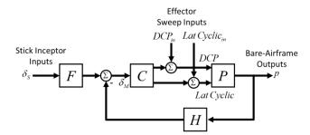
Figure 2. Top level V-280 closed-loop block diagram (lateral axis, hover).
