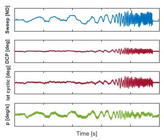
Figure 3. Piloted lateral stick sweep in hover shows that DCP and Lateral Cyclic (at the rotor head) are highly-correlated.
