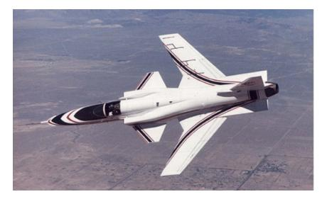
Fig. 17 X-29A forward-swept wing fly-by-wire demonstrator.
