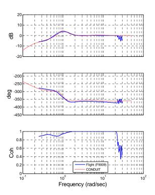
Figure 7 – ACVH longitudinal ground speed disturbance rejection response comparison between analysis and flight
