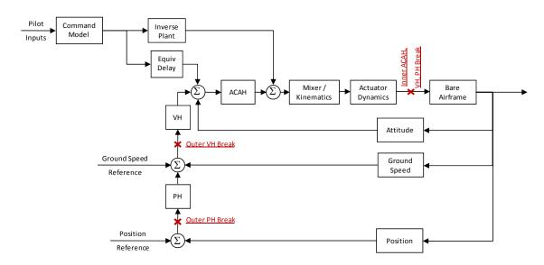
Figure 13 – Inner and outer loop break locations for stability margin calculations
