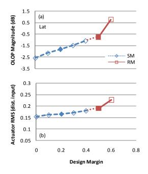
Figure 18 – Lateral OLOP and actuator RMS (for disturbance inputs) results (flight cases filled)
