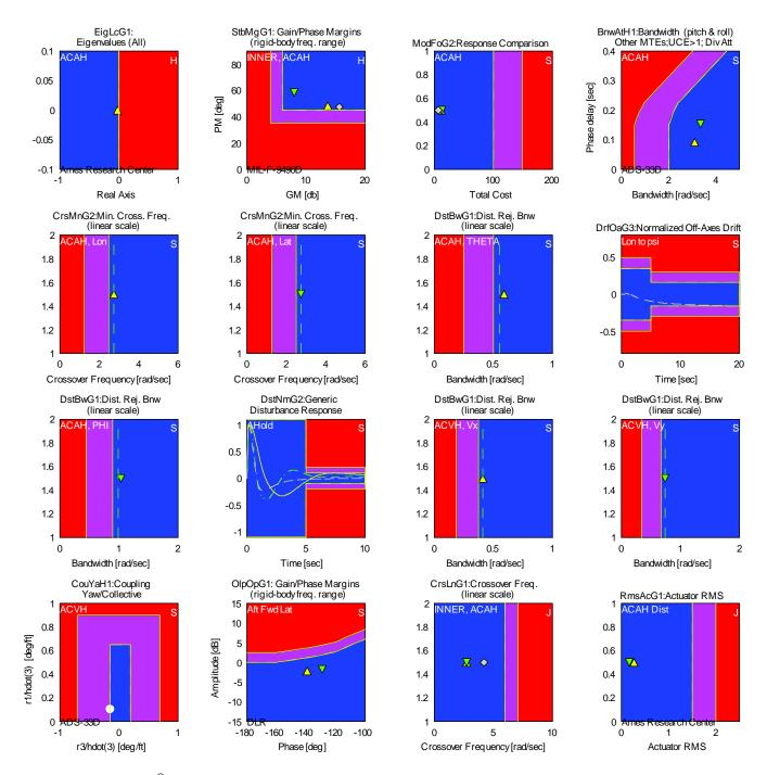
Figure 10 – CONDUIT<sup>®</sup> HQ Window for 0.2 Design Margin case of standard margins family of results
