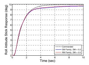
Figure 20 - Roll attitude response to step input at stick
