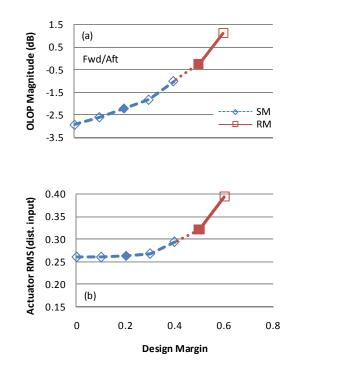
Figure 14 – Longitudinal OLOP and actuator RMS (for disturbance inputs) results (flight cases filled)
