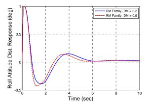
Figure 21 – Roll attitude response to unit disturbance
