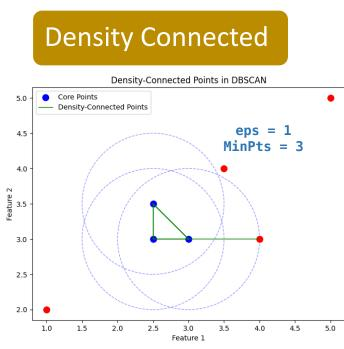
p and q are said to be **density-connected** w.r.t. eps and MinPts if there exists a point v such that:
