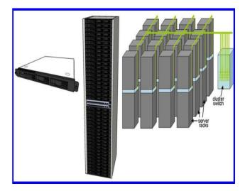
**FIGURE 1.1:** Architecture of WSC; Typical elements in warehouse-scale systems: 1U server (left), rack with Ethernet switch (middle), and diagram of a small cluster with a cluster-level Ethernet switch/router (right).
