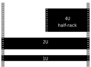
FIGURE 1.2: Different height of servers placed in a rack
