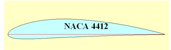
Figure 21. Shape of NACA 4412 airfoil
