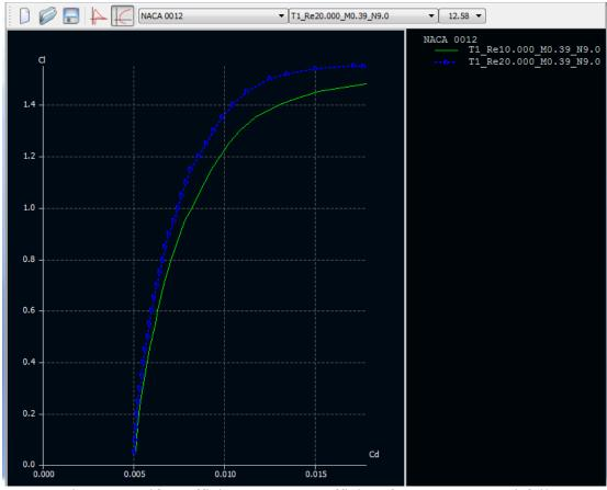
Figure 23. Lift coefficient vs Drag coefficient for NACA 0012 airfoil
