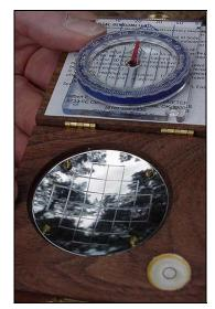
Figure 19: Spherical Densiometer
