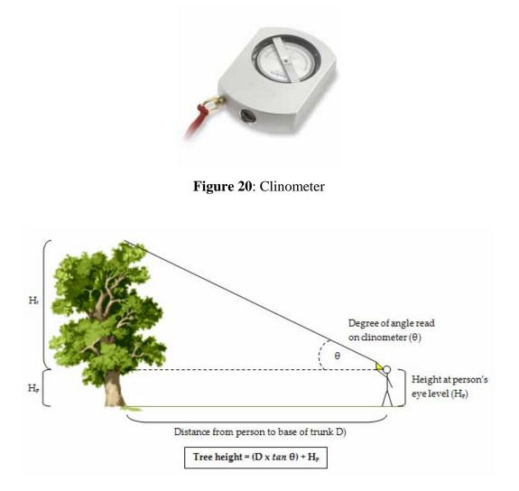
Figure 21: How to measure the height of a tree on a flat surface.
