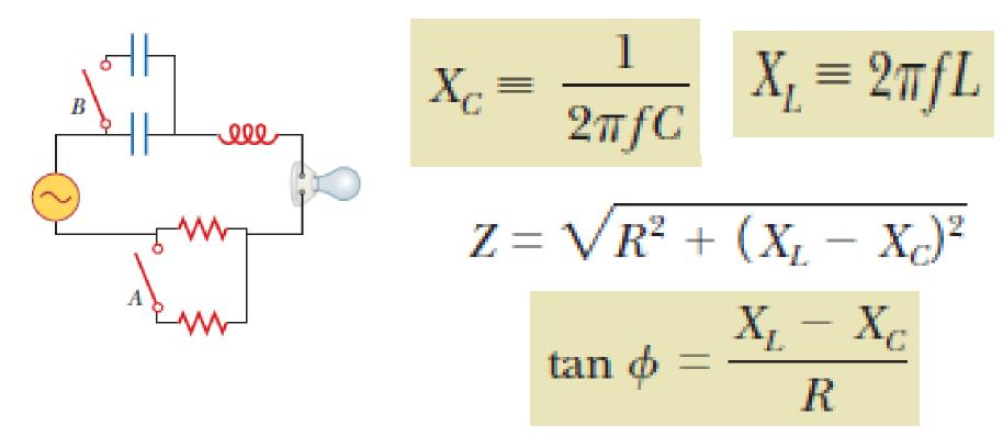
3. Suppose *XL* >*XC* in Fig. If switch A is left open and switch B is closed, what happens to the phase angle? (a) It increases. (b) It decreases. (c) It doesn't change.
