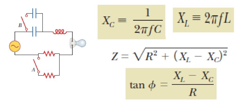
1. If switch A is closed in Fig, what happens to the impedance of the circuit? (a) It increases. (b) It decreases. (c) It doesn't change
