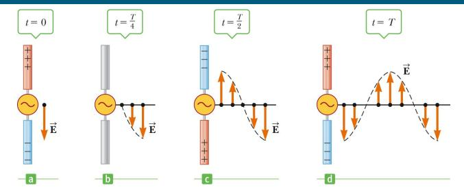
•Two rods are connected to an ac source, charges oscillate between the rods (a).
