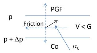
Wind at angle  $\alpha_0$  to isobars ("cross isobaric flow angle").
