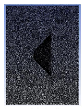
Figure 2.14 - Meshed 45 degree blunt nose cone
