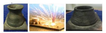
Figure 1.5 - Arc-based deposition [4]
