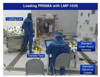
Figure 3: Equipment used to handle LMP-103S (Beckel & Dinardi)
