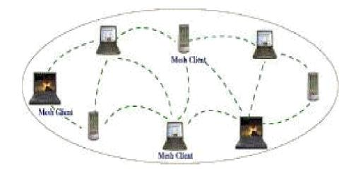
*Figure 3*. An example of Client Mesh Architecture. Adapted from *Wireless mesh networks: a survey* (p. 448), by I. Akyildiz, X. Wang, 2004, Bridgewater, NJ: Elsevier B.V. Copyright 2004 by Elsevier B.V.
