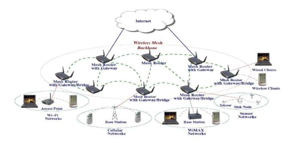
*Figure 2*. An example of Infrastructure Mesh Architecture. Adapted from *Wireless mesh networks: a survey* (p. 448), by I. Akyildiz, X. Wang, 2004, Bridgewater, NJ: Elsevier B.V. Copyright 2004 by Elsevier B.V.
