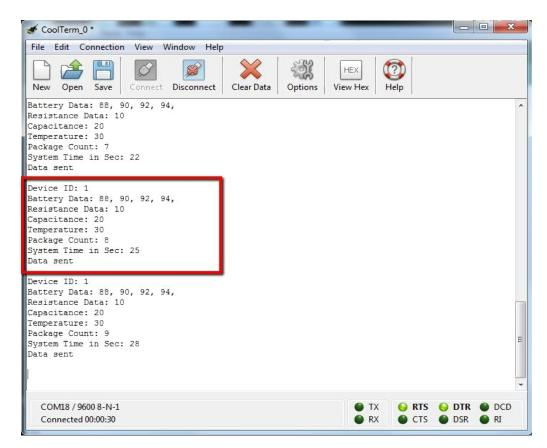
Figure 11. Router XBee transmitted data to other devices on same network
