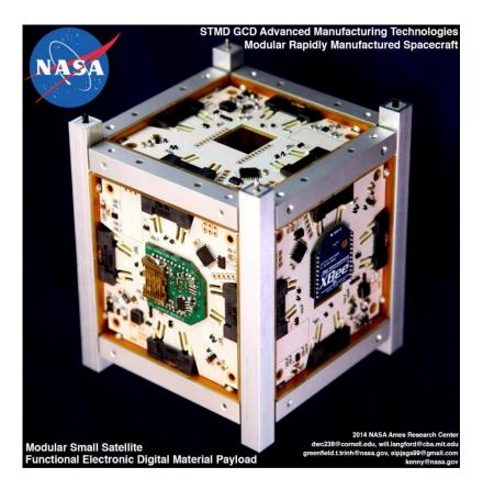
Figure 16. The Modular Rapidly Manufactured Small Satellite (MRMSS) prototype image
