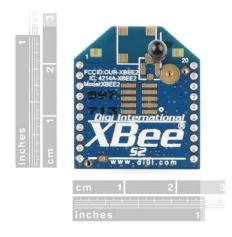
*Figure 5*. An example of XBee Series 2 image. Adapted from XBee 2mW wire antenna, In *Sparkfun*, n.d., Retrieved April 15, 2015, from <u>https://www.sparkfun.com/products/10414</u>.
