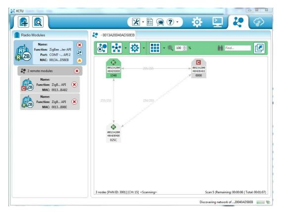
Figure 9. XCTU Mesh Network successful connection with three XBee Series 2
