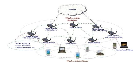
*Figure 4*. An example of Hybrid Mesh Architecture. Adapted from *Wireless mesh networks: a survey* (p. 449), by I. Akyildiz, X. Wang, 2004, Bridgewater, NJ: Elsevier B.V. Copyright 2004 by Elsevier B.V.
