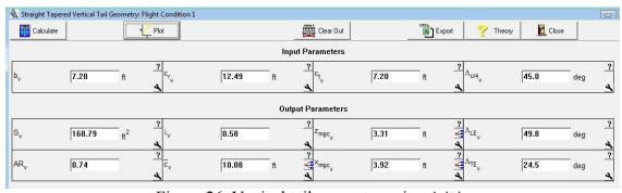
Figure 26. Vertical tail geometry using AAA
