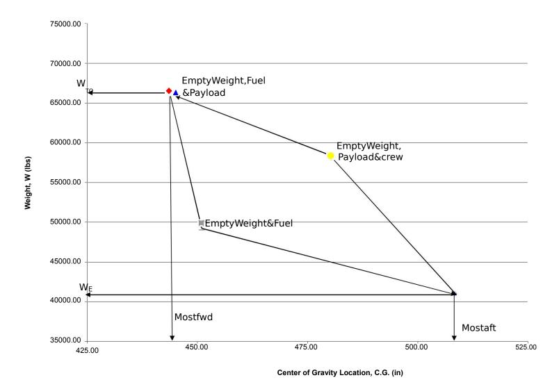
Figure 36. Center of Gravity excursion diagram
