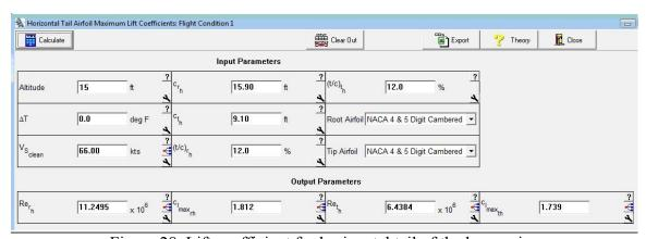
Figure 28. Lift coefficient for horizontal tail of the hoverwing
