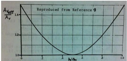
Figure 41. Effective value of vertical tail aspect ratio
