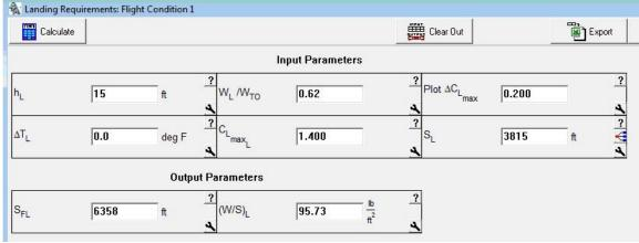
Figure 9. AAA calculation for landing requirement
