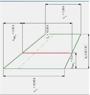
Figure 27. Vertical tail planform using AAA
