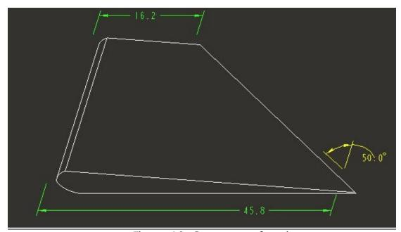
Figure 19. Geometry of a wing
