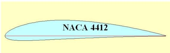
Figure 21. Shape of NACA 4412 airfoil
