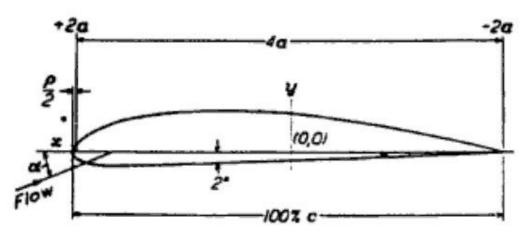
Figure 16. Geometry of Clark Y airfoil [6]
