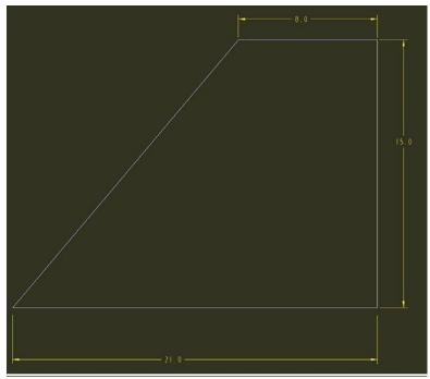
Figure 20. Geometry of a winglet
