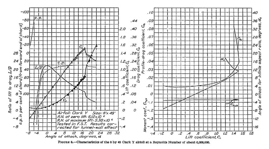
Figure 17. Lift coefficient vs Drag coefficient curve for Clark Y airfoil [6]
