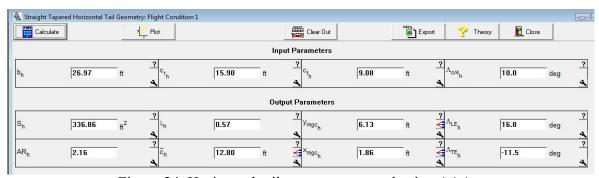
Figure 24. Horizontal tail geometry tapered using AAA
