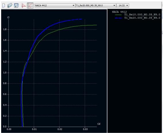
Figure 22. Lift coefficient vs Drag coefficient for NACA 4412 airfoil
