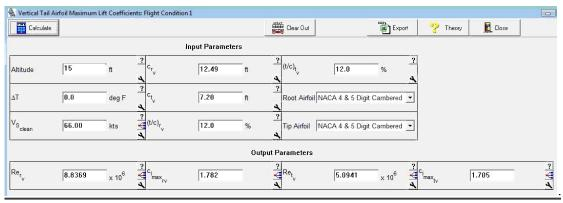
Figure 29. Lift coefficient for vertical tail of the hoverwing
