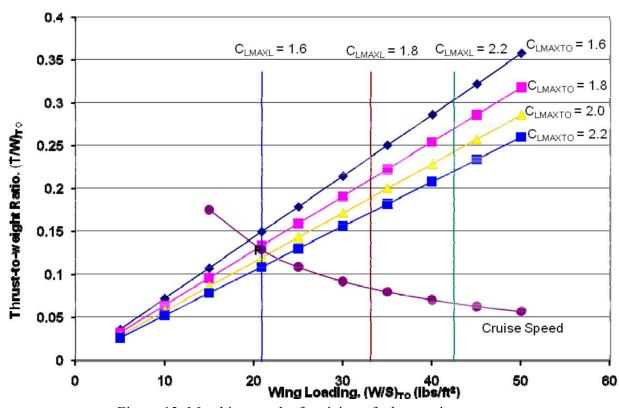
Figure 12. Matching results for sizing of a hoverwing
