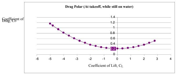
Figure 46 Drag Polar (At takeoff, while still on water)
