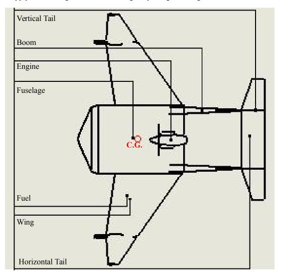
Figure 34. Location of centre of gravity in X-direction
