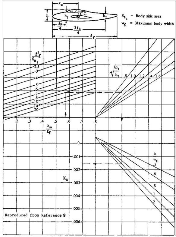
Figure 42. Factor accounting for wing-fuselage interference with directional stability [11]
