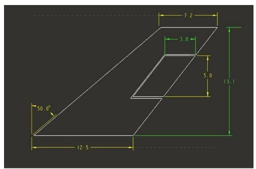
Figure 30. Geometry of a vertical stabilizer
