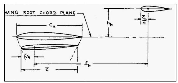
Figure 38. Geometric parameters for horizontal tail location
