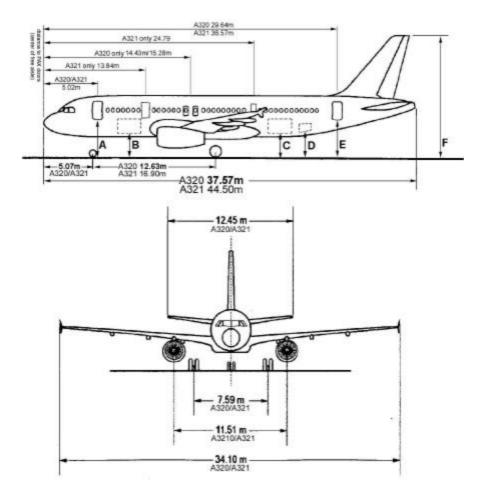
Figure 12. Airbus A320NEO aircraft configuration (Airbus Commerial Aircraft, n.d.)
