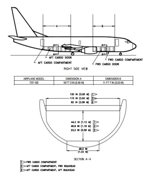
Figure 47. Side view of fuselage with cargo compartment visible (Boeing Commercial Airplanes, 2013)
