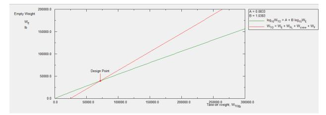
*Figure 20.* W<sub>e</sub> vs. W<sub>to</sub> of 2 turbojet engine fuel-powered aircraft with ideal design point of W<sub>to</sub>=71,635.9 lbs and W<sub>e</sub>=39,775.9 lbs
