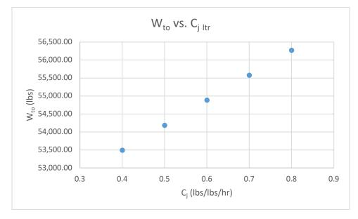
Figure 28. Takeoff Weight vs. Specific Fuel Consumption during Loiter
