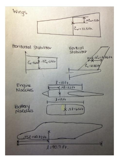
Figure 61. c.g. for various aircraft components
