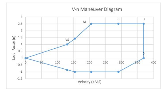
Figure 87. V-n Maneuver Diagram
