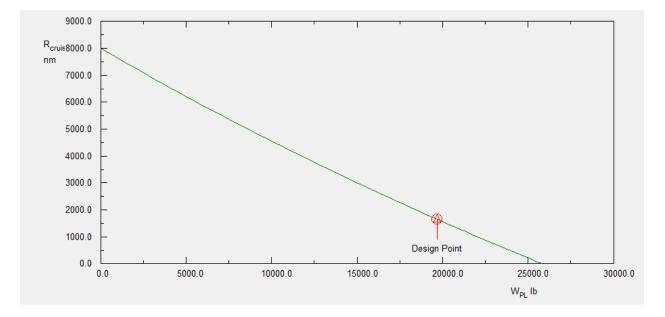
*Figure 30.* Range vs. Payload with design point  $W_{pl}$ =19,630.6 lb and  $R_{cr}$ =1,638.7 nm for fuel-powered aircraft
