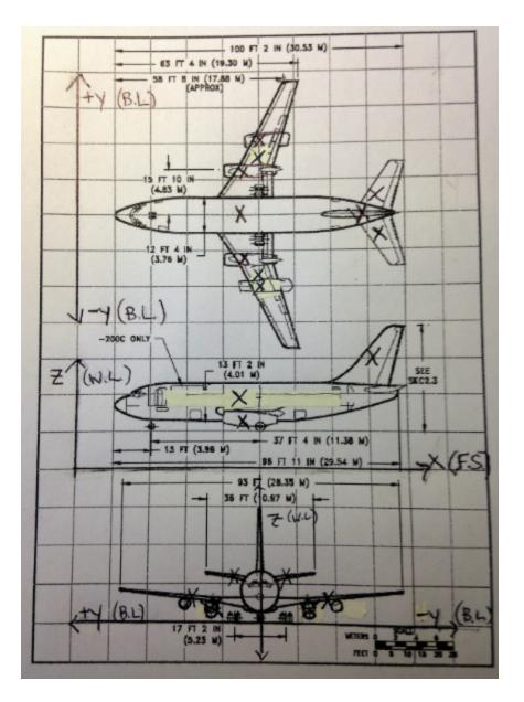
Figure 62. c.g. location for each component on the aircraft
