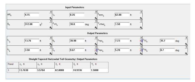
Figure 57. Horizontal Tail Geometry Calculations by AAA
