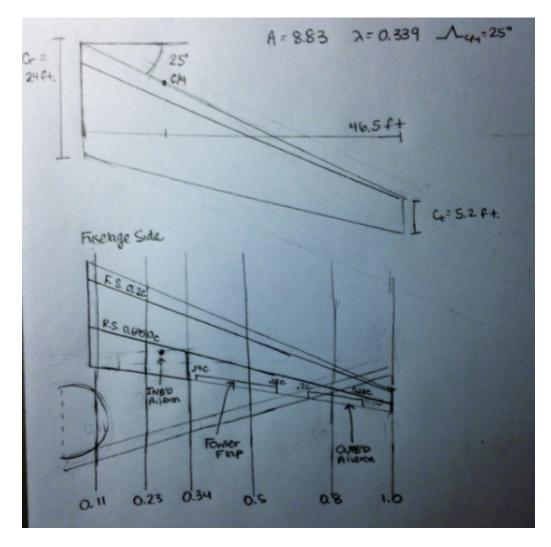
Figure 55. Wing Planform: flap and lateral control layout
