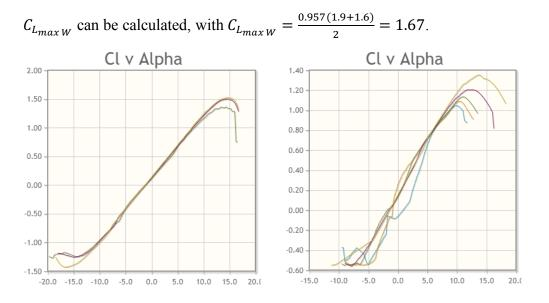
Figure 52. Clvs. angle of attack for maximum lift coefficient at root and midspan
