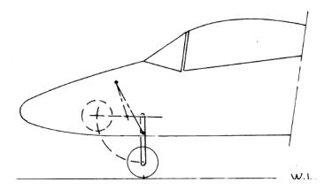
Figure 72. Nose gear retraction
