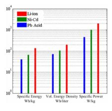
compared to Ni-Cd and Pb-acid, at \$0.42 and \$0.28, respectively, they have the highest energy density offered, which means they are the smallest in both volume and weight for the amount of energy stored. Figure 5 illustrates the capabilities of Li-ion batteries' specific energy, volumetric energy density, and specific power, and compares them against
