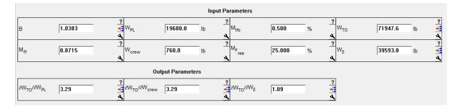
Figure 21. Takeoff weight sensitivities calculated by AAA for fuel-powered aircraft
