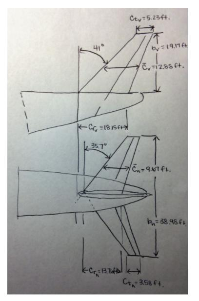
Figure 56. Empennage Configuration (units in feet)
