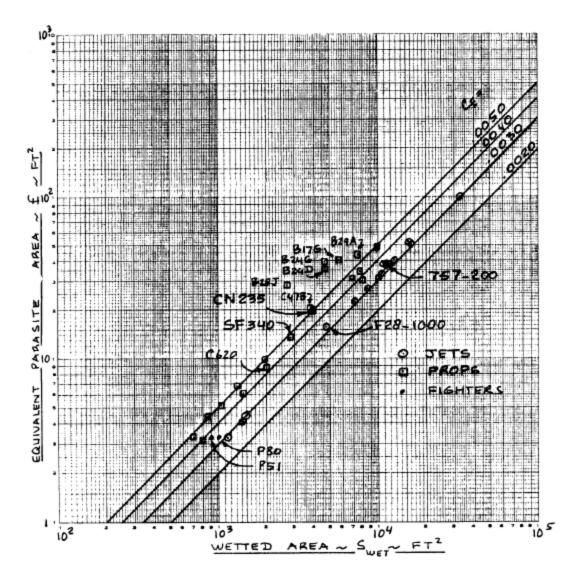
Figure 81. Wetted area vs. equivalent parasite area
