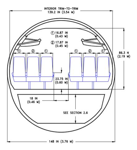
Figure 44. Front view of the fuselage (Boeing Commercial Airplanes, 2013)
