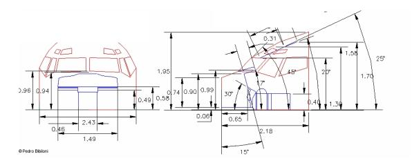
*Figure 41.* Front and side 3-D view of cockpit. Dimensions in meters (*Boeing Commercial Airplanes*, 2013)
