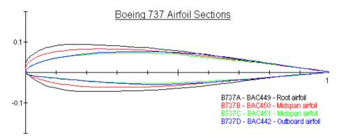
*Figure 51*. Boeing 737 Airfoil selections schematic (*Aircraft Technical Data and Specifications: Boeing* 737-100/200, 2017)
