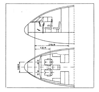
*Figure 40.* Side and top-down view of cockpit. Dimensions in meters (*Boeing Commercial Airplanes*, 2013)
