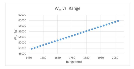
Figure 26. Takeoff Weight vs. Range
