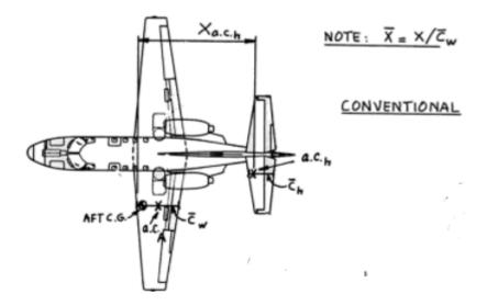
Figure 76. Geometric quantities for aircraft calculations
