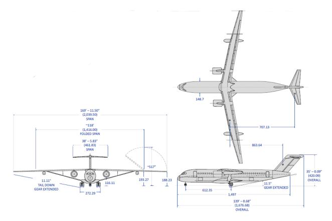
*Figure 15.* SUGAR Volt 765-096 RevA aircraft configuration (Bradley & Droney, Subsonic Ultra Green Aircraft Research: Phase II- Volume II- Hybrid Electric Design Exploration, 2015)
