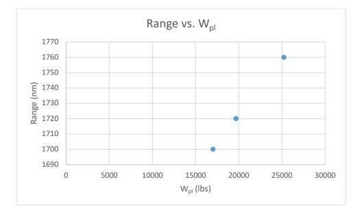
Figure 29. Range vs. Payload
