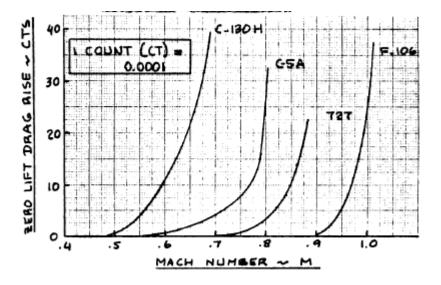
Figure 82. Typical Compressibility Drag Behavior
