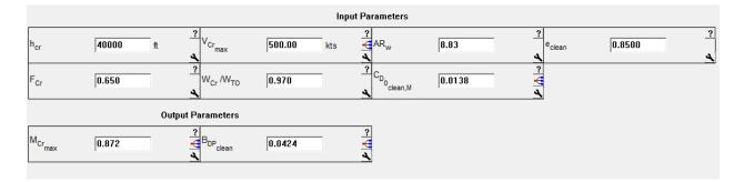
Figure 35. AAA results of cruise speed requirement sizing
