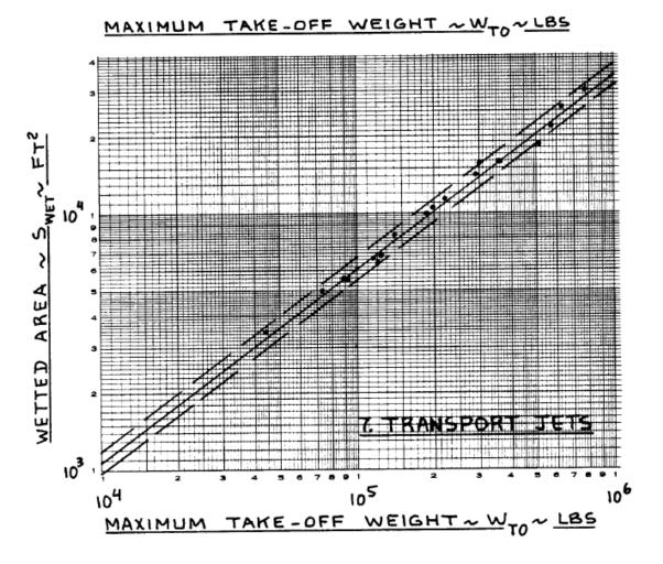
*Figure 80.* Maximum takeoff weight vs. wetted area for jet transports Using the plot below, the equivalent parasite area of the HTA is approximately 22 ft<sup>2</sup>.
