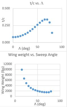
Figure 50. Plots of t/c and  $W_w$  vs.  $\Lambda$
