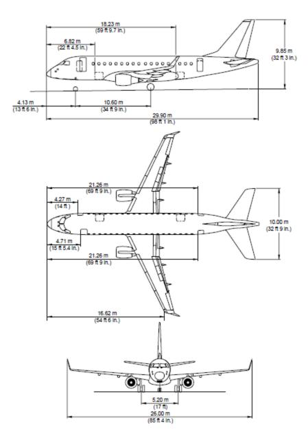
Figure 13. Embraer ERJ-170-100 aircraft configuration (Jane's All the World's Aircraft, 2013)
