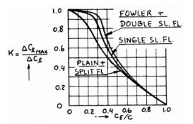
Figure 53. Effect of Flap Chord Ratio and Flap Type on K
