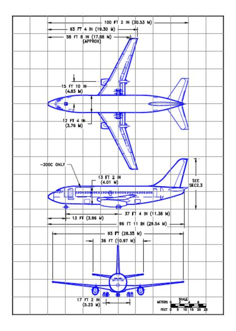
Figure 11. Boeing 737-200 aircraft configuration. (Boeing Commercial Airplanes, 2013)
