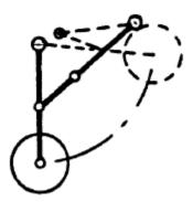
Figure 73. Stick Diagram for main gear retraction
