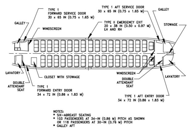
Figure 43. Top down view of the fuselage (Boeing Commercial Airplanes, 2013)
