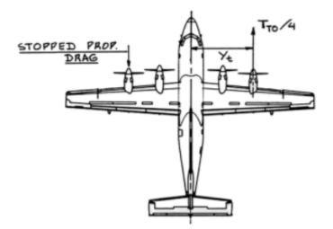
Figure 79. Geometry for one engine out  $V_{mc}$  calculations
