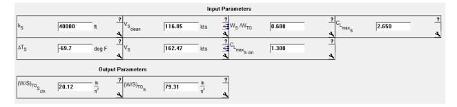
Figure 31. AAA results of stall speed sizing
