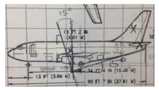
Figure 71. Landing gear and strut placement
