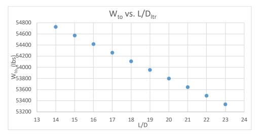
Figure 24. Takeoff Weight vs. L/D for Loiter
