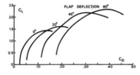
Figure 83. Low speed polars for transport
