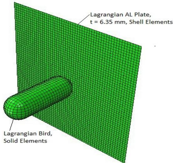
**Figure 14: Bird model setup (Lagrangian Formulation)**
