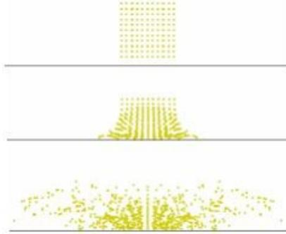
**Figure 5: Soft body impact in SPH formulation [22]**
