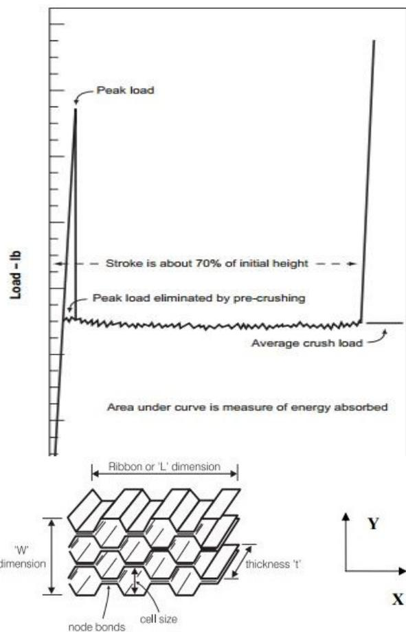
Figure 8: Load-Displacement Curve of Out-of-Plane Compression of Honeycomb Core [36]
