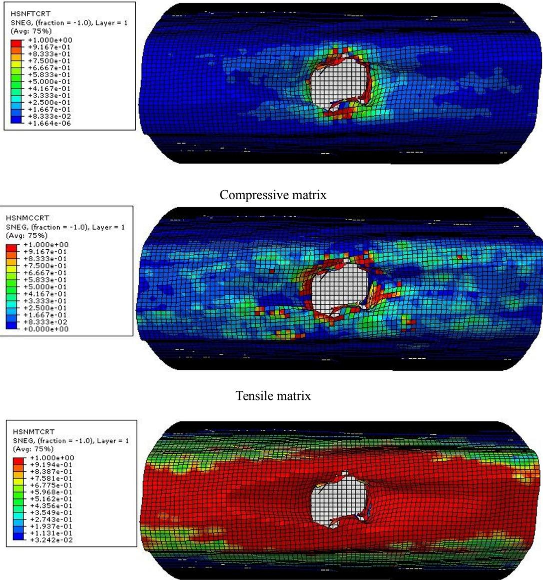
Figure 26: Composite top skin failure modes (ACG-1 core and CFRP skins)
