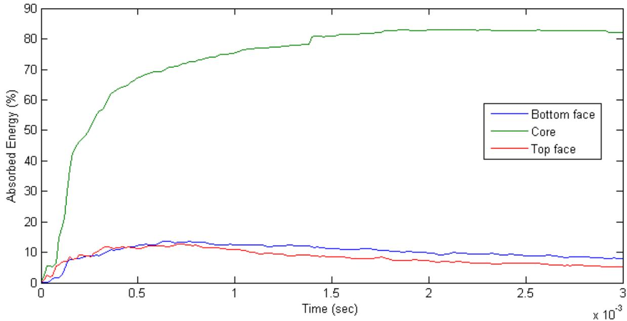
Figure 34: Kinetic energy absorbed vs. Time (ACG-1 core and CFRP skins)
