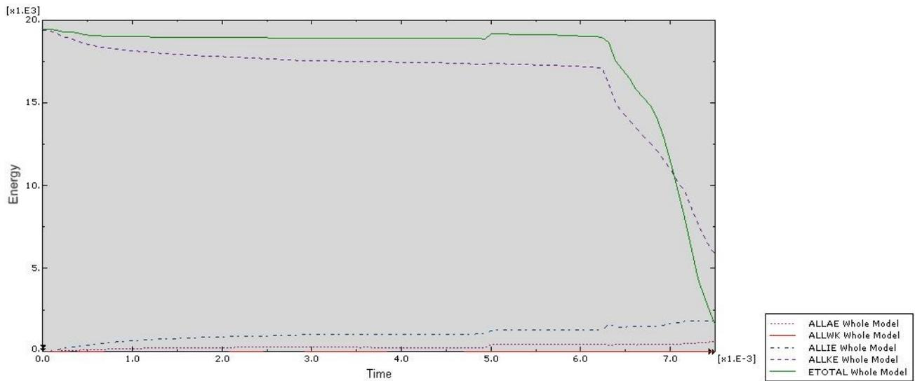
Figure 28: Energy balance chart for the wing leading edge (CFRP skins and ACG-1 core)
