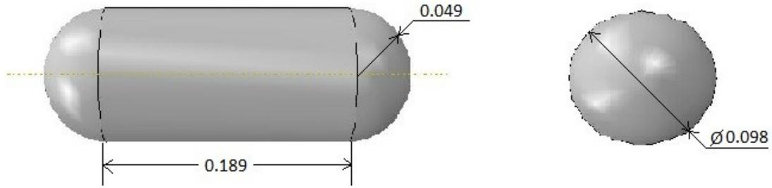
**Figure 13: Bird geometry (All dimensions are in meters)**
