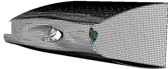
**Figure 25: Bird strike event at different time interval (ACG-1 core and CFRP skins)**
