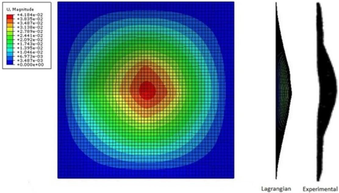
Figure 16: Displacement contours of Aluminum plate (Lagrangian Method), at  $V = 150$  m/s
