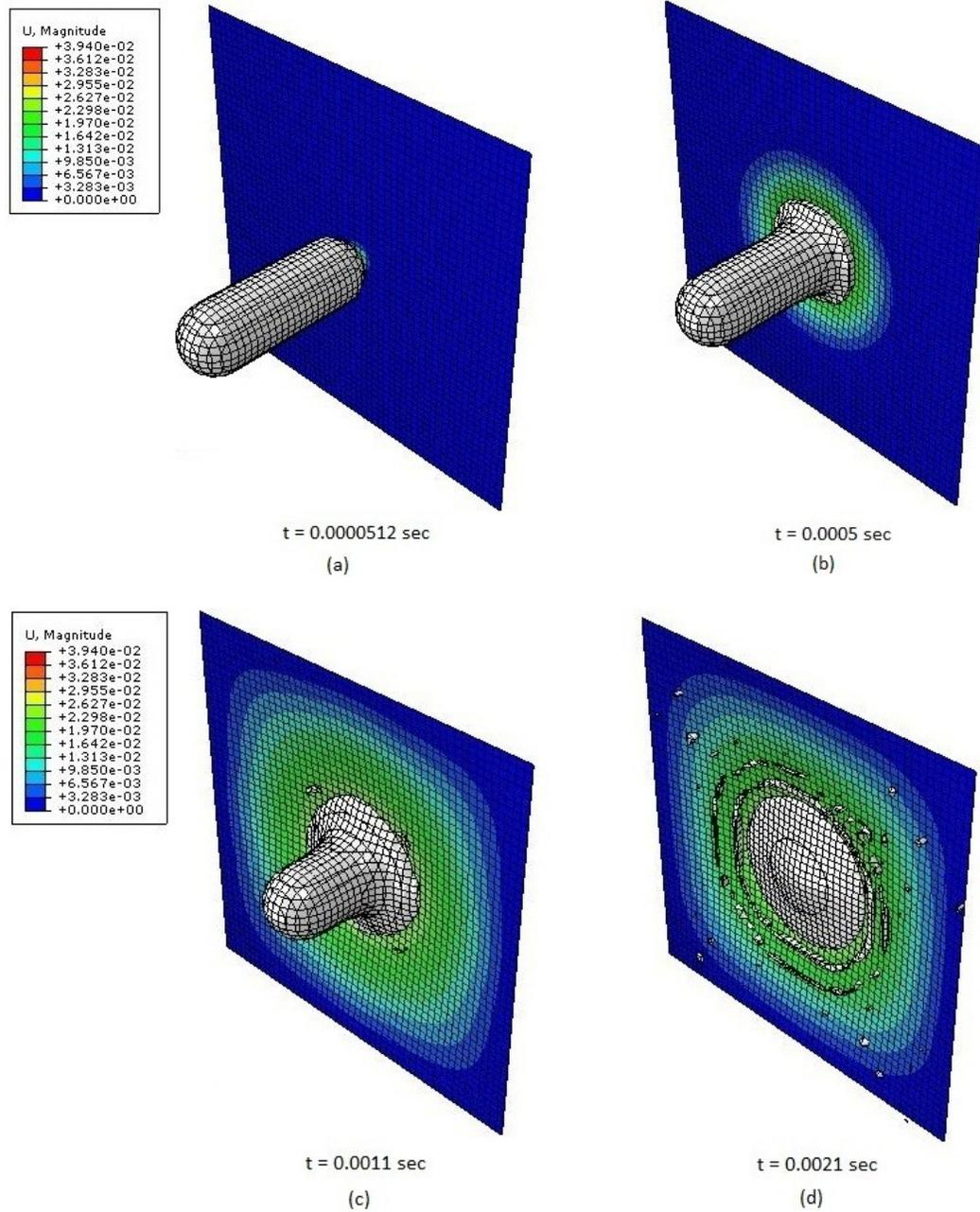
**Figure 18: Bird Impact at various time interval, at  $V = 150 \text{ m/s}$**
