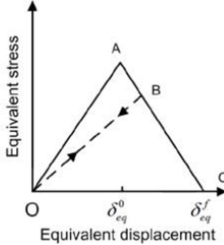
Figure 10: Equivalent Stress-Displacement Diagram [4]
