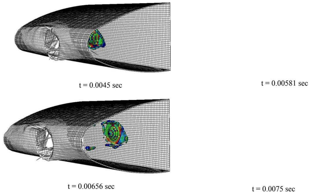
**Figure 23: Bird strike event at different time interval (ACG-1/4 core and CFRP skin)**
