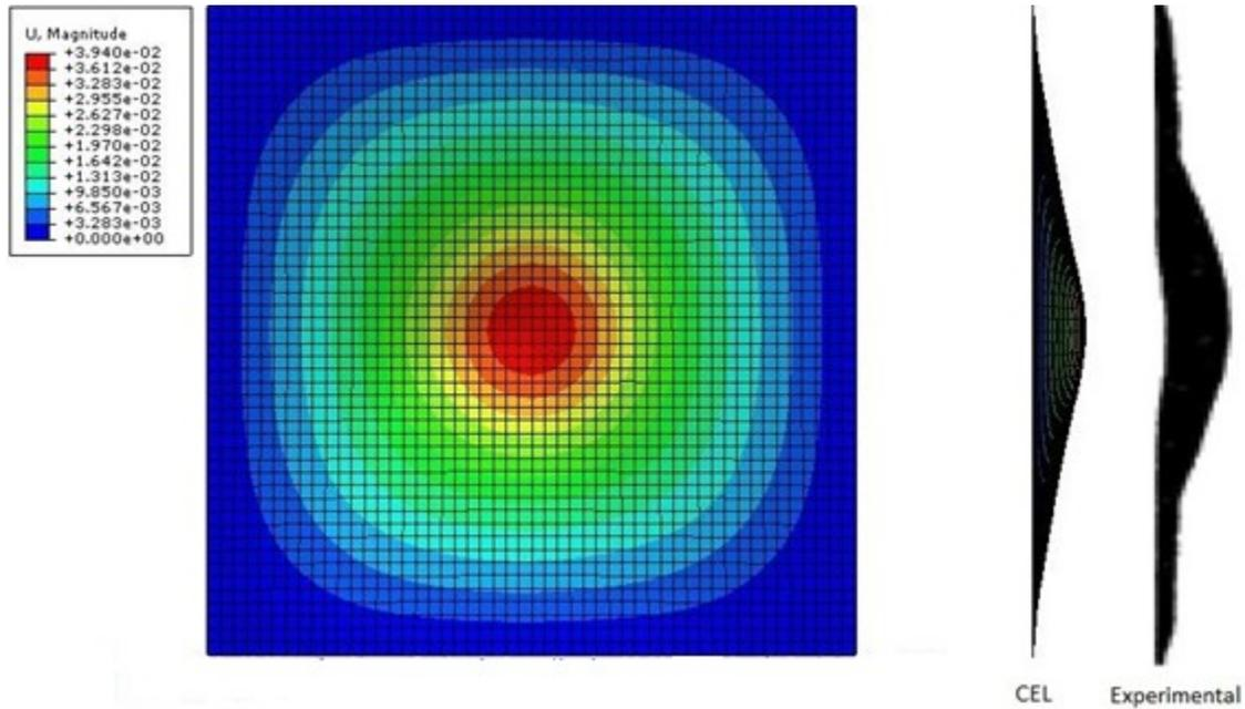
Figure 17: Displacement contours of Aluminum plate (CEL Method), at  $V = 150$  m/s
