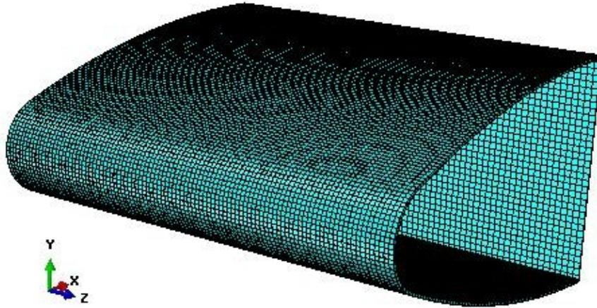
Figure 9: Wing Leading Edge Finite Element Mesh
