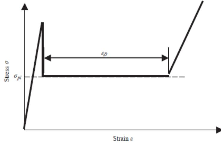
Figure 12: Schematic Stress-Strain Curve for Honeycomb [39]
