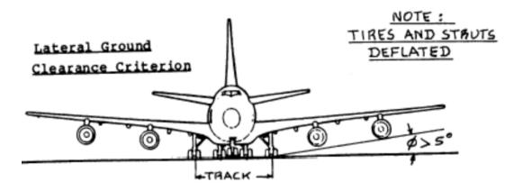
Figure 8.12: Lateral ground clearance criterion for tricycle gear
