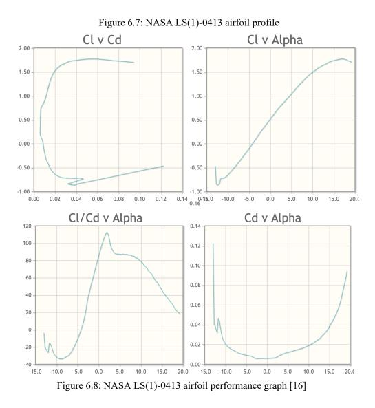
From Figure 6.8, the graph of  $C_L$  versus  $\alpha$  for the NASA LS airfoil show that the proposed wing tip airfoil can produce  $C_L$  of 1.70 at an angle-of-attack of 19.25 degrees. Substantial improvement in  $c_{l max}$  for LS airfoils throughout the reynolds number range were seen when compared to the NACA 4 and 5 digit airfoils and 65 series airfoils
