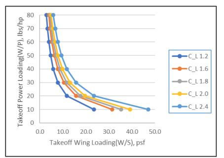
Figure 3.3: Effect of take-off wing loading and maximum take-off lift coefficient on take-off power loading
