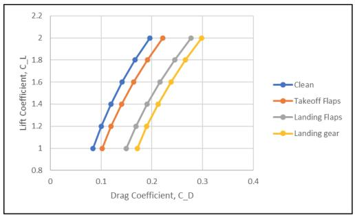
Figure 11.2: Cruise, takeoff and landing drag polar
