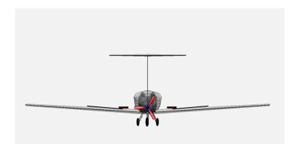
Figure 8.14: Front view of the proposed aircraft with landing gear disposition
