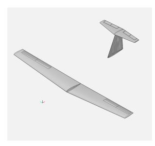
Figure 7.6: Isometric view of empennage planform with respect to wing planform
