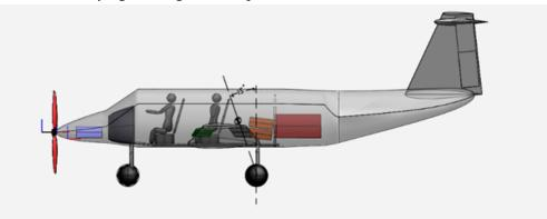
Figure 8.7: Longitudinal tip-over criterion for the proposed aircraft
