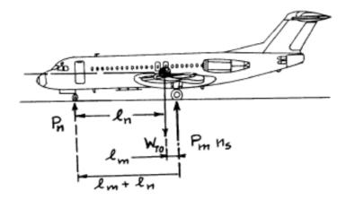
Figure 8.5: Geometry for Static load tricycle gear
