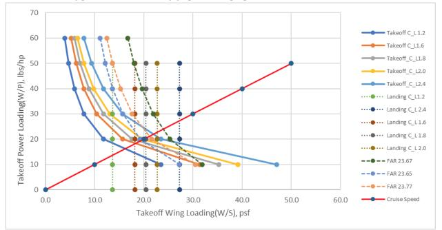
Figure 3.15: Performance sizing graph of manual calculations
