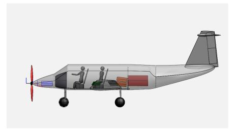
Figure 12.2: Side view of the proposed aircraft
