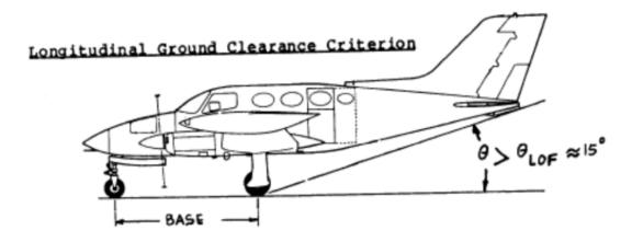
Figure 8.10: Longitudinal ground clearance criterion for tricycle gear [1]
