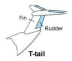
Figure 4.6: T-tail configuration
