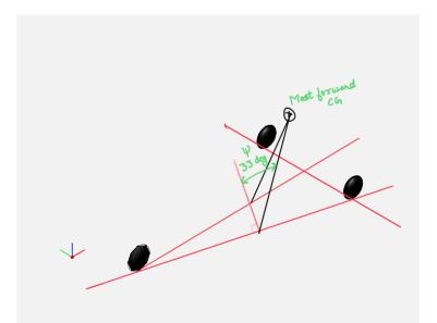
Figure 8.9: Lateral Tip-over criterion for the proposed aircraft
