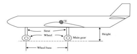
Figure 8.1: Landing Gear Parameters
