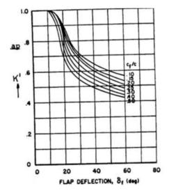
Figure 6.12: Effect of thickness ratio and flap chord ratio on  $c_{1_{\delta_f}}$
