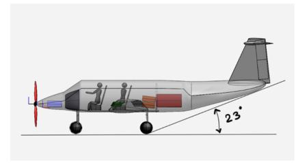
Figure 8.11: Longitudinal ground clearance criterion for the proposed aircraft
