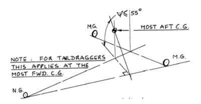
Figure 8.8: Lateral tip-over criterion
