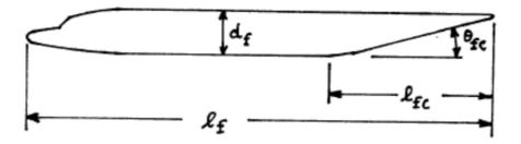
Figure 5.6: Definition of geometric fuselage parameters [1]
