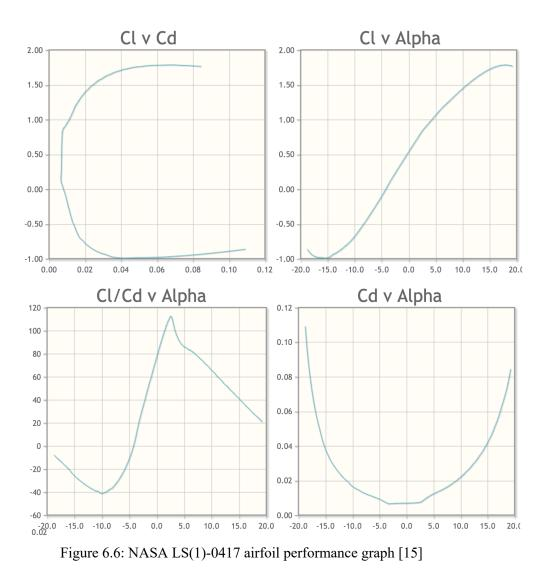
From Figure 6.6, it can be noted that the maximum lift coefficient increases with an increase in Reynold's number and note that the actual calculations of Reynolds number will be carried out in the next sections. The graphs of  $C_L$  versus  $\alpha$  for the NASA LS-0417 airfoil show that the proposed wing root airfoil can produce  $C_L$  of 1.76 at an angle-of-attack of 19.25 degrees.
