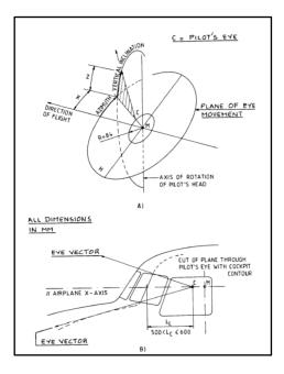
Figure 5.3: Radial eye vector's definition [1]
