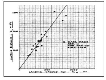
Figure 3.6: Relation between ground run and landing distance [1]
