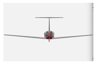
Figure 4.5: Low-wing design of the proposed aircraft
