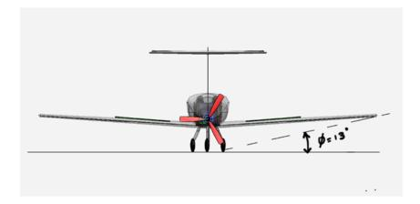
Figure 8.13: Lateral ground clearance criterion for the proposed aircraft
