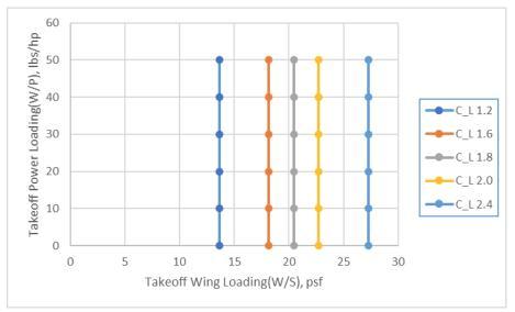
Figure 3.7: Allowable wing loading to meet landing distance requirement
