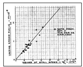
Figure 3.5: Effect of square of stall speed on landing ground run [1]
