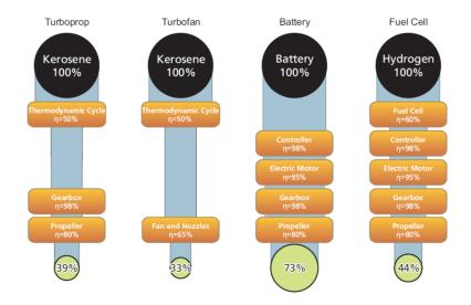
Figure 2.2: Different propulsion system efficiencies [11]
