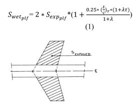
Figure 11.1 Exposed Planform Definition
