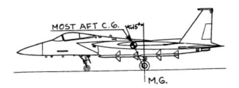
Figure 8.6: Longitudinal tip-over criterion for tricycle gear
