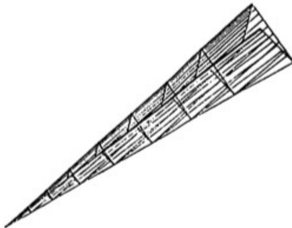
**Figure 2. Optimized inviscid waverider at Mach 10; a caret wing [5]**
