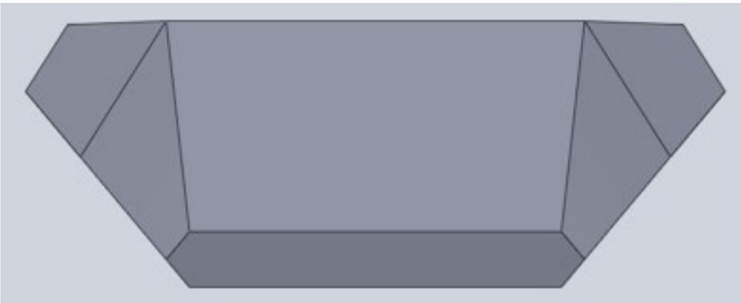
**Figure 32. Bow View of Proto-Waverider by Loft Method**
