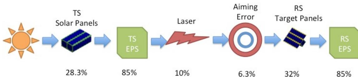
**Figure 12: End-to-End Efficiency**
