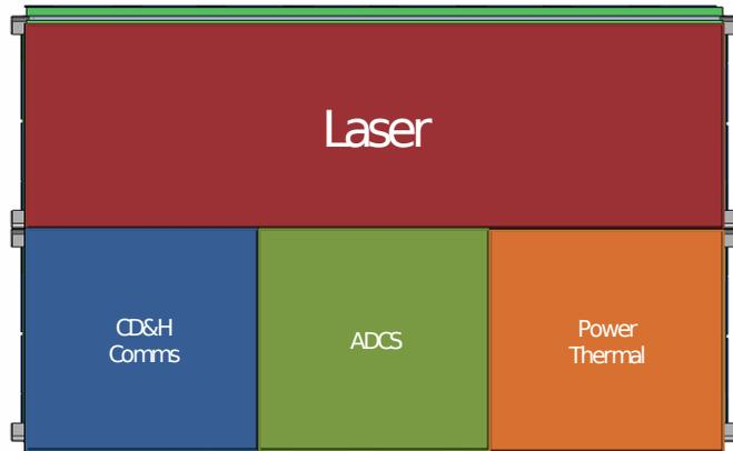
**Figure 9: TS Subsystem Volume Allocation**
