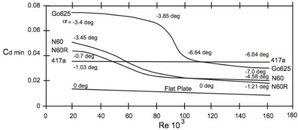
Figure 25: Minimum coefficient of drag vs. Reynolds for Schmitz's five airfoils. [7]
