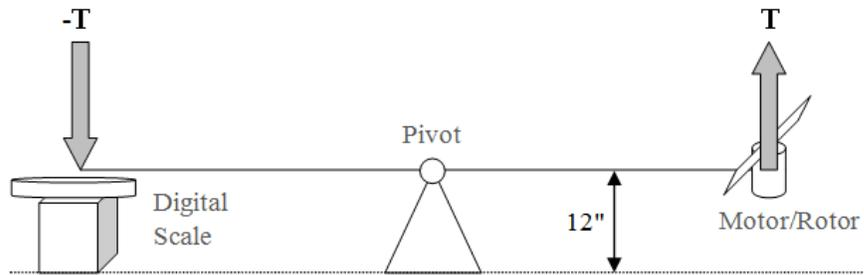
Figure 48: Free body diagram of lever apparatus to measure thrust. All rotors tested were 12" above the surface.
