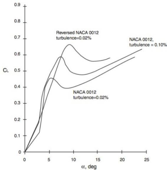
Figure 26a: Coefficient of lift vs. angle of attack for NACA 0012 with varying turbulence and orientation. [7]
