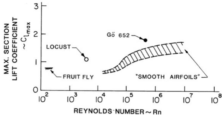
Figure 27: Compilation of lift coefficients at increasing Reynolds numbers.
