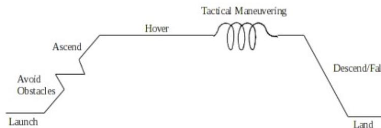
**Figure 5: Flight profile for optimum objectives.**
