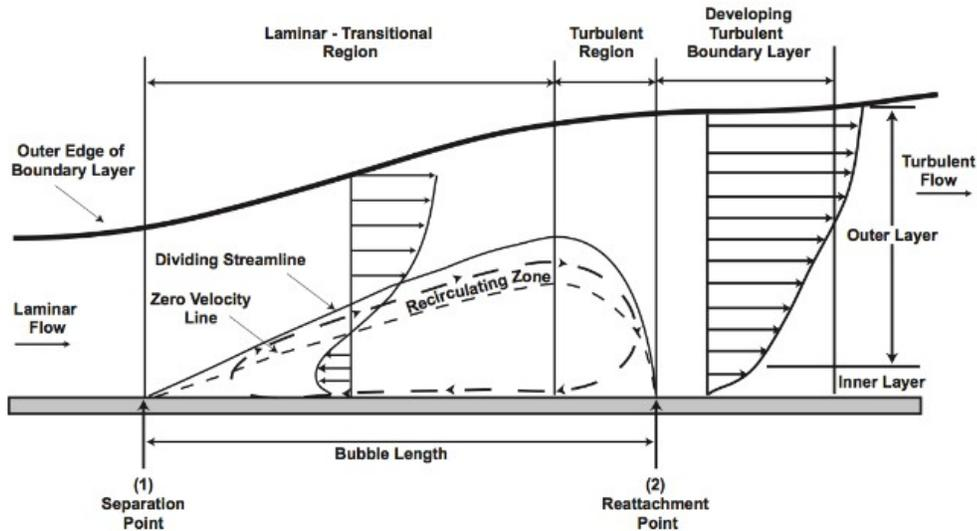
Figure 22: Transitional boundary layer showing separation bubble and turbulent reattachment. [7]
