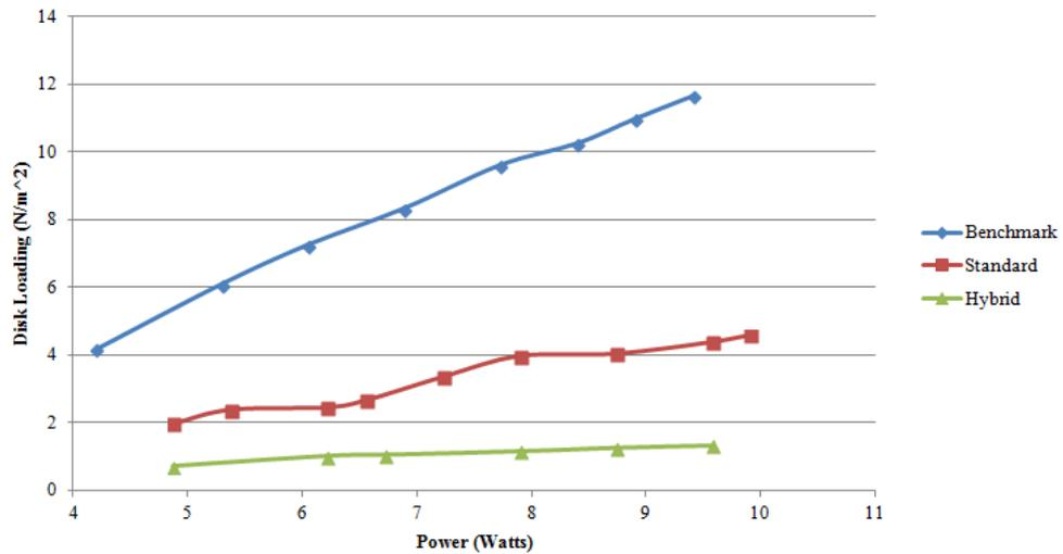
Figure 50: Disk loading on tested rotors for increasing values of electrical power.
