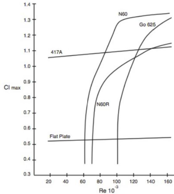
Figure 24:  $C_{l\ max}$  vs. Reynolds number for the five airfoils examined by Schmitz. [7]
