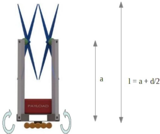
**Figure 12: Arms rotate upwards and inwards as illustrated. The relay/payload is shown in red and batteries in orange.**
