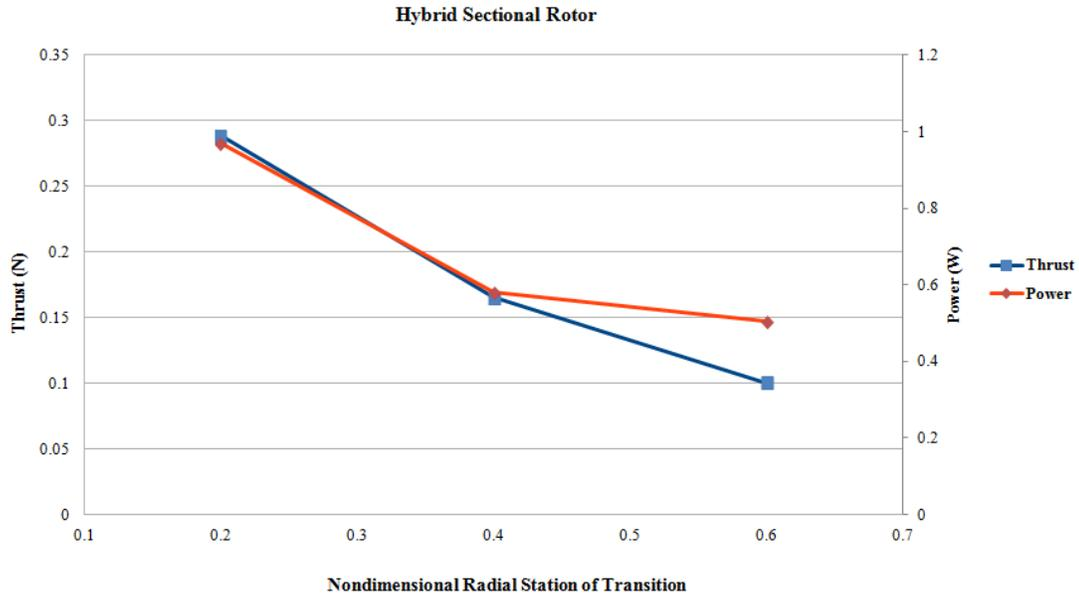
Figure 34: Thrust vs. radial location of geometric transition.
