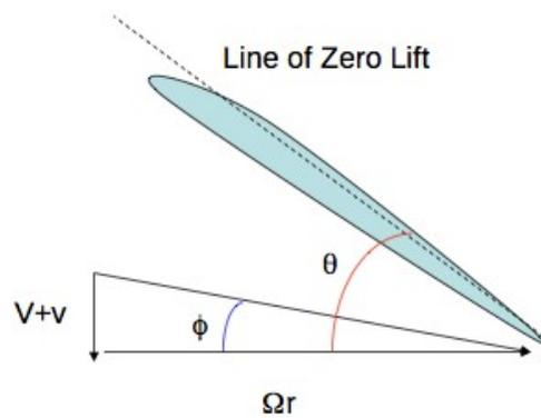
Figure 30: Inflow velocity, pitch angle, and inflow angle angle of attack. [8]
