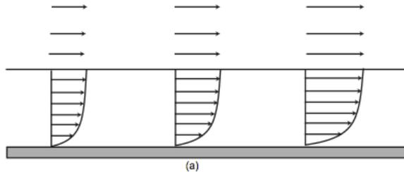
**Figure 20a: Laminar boundary layer. [7]**
