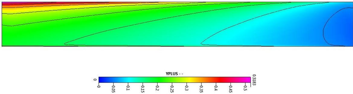
**Figure 39: Y+ values on the upper surface of standard blade at 1000 RPM.**
