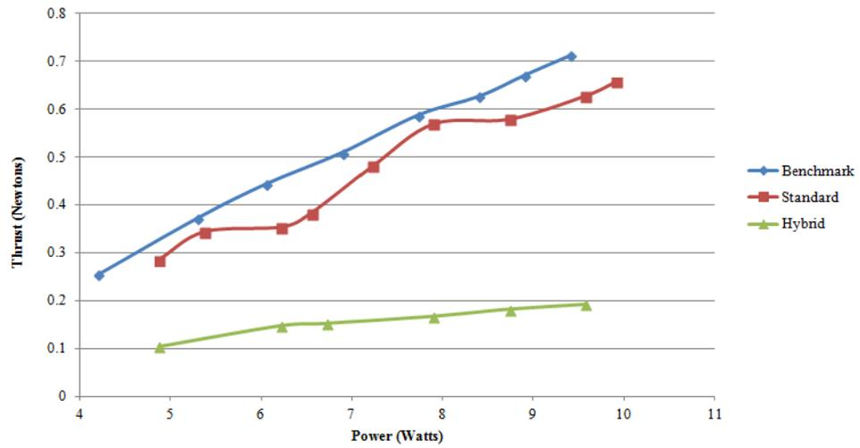
Figure 49: Measured thrust for increasing input power for the benchmark, standard, and hybrid rotors.
