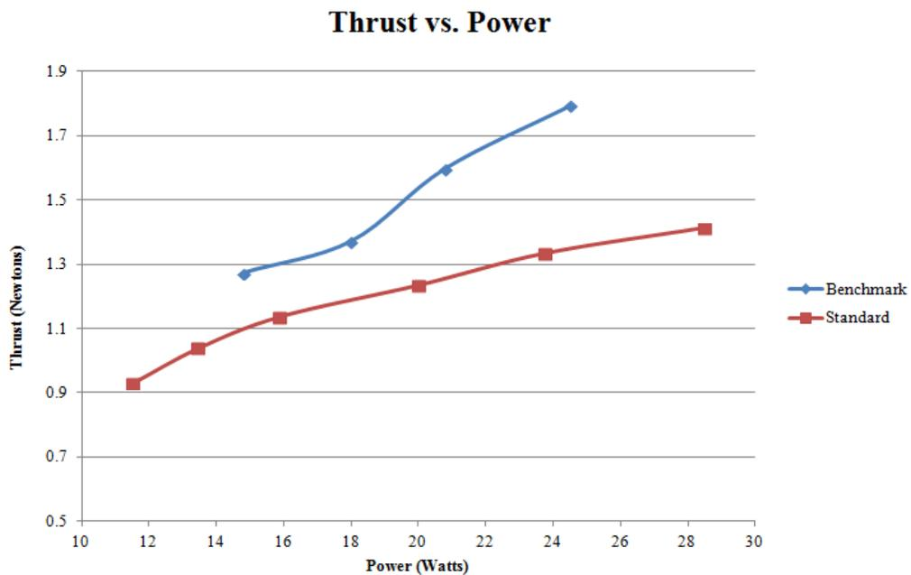
Figure 51: Performance comparison between the benchmark and standard rotors at higher rotational speeds.
