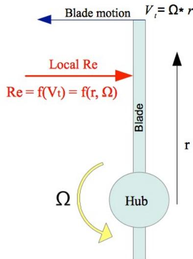
Figure 18: Local Reynolds number as a function of radial location.
