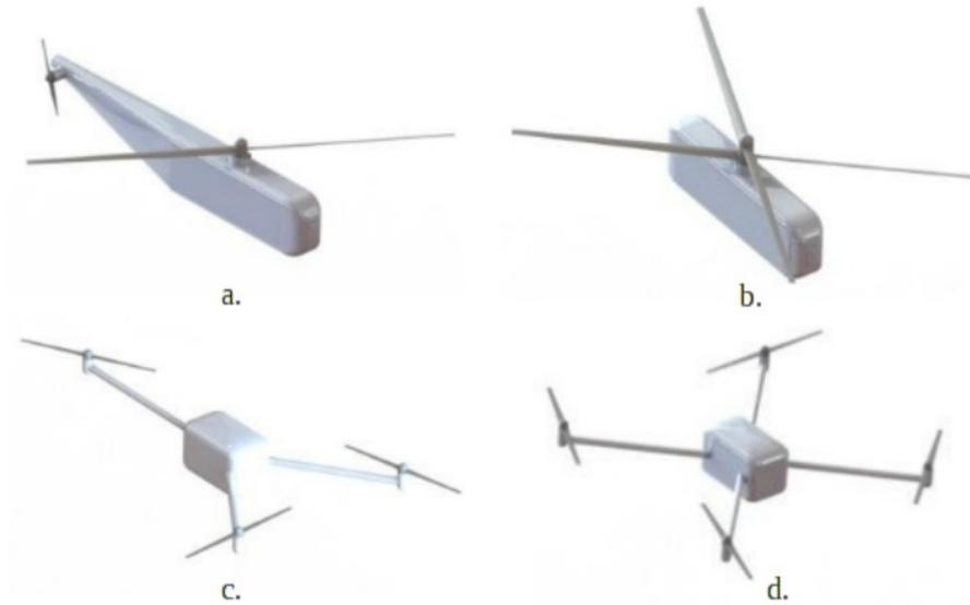
**Figure 6a-d: Possible rotorcraft configurations: a Conventional Helicopter, b. Coaxial, c. Trirotor 'Y', d. Quadrotor**
