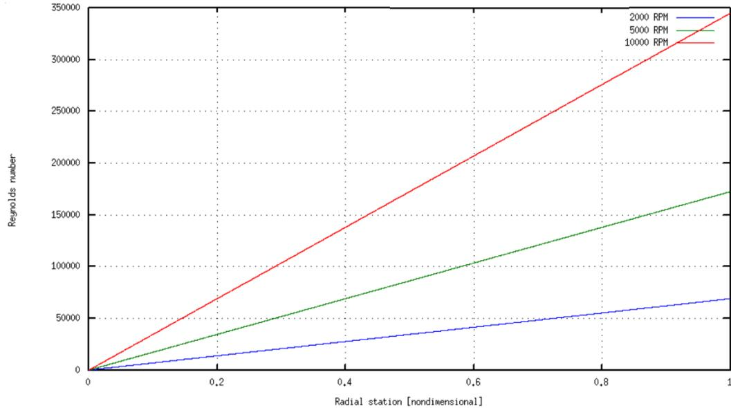
Figure 19: Reynolds number vs. radial location for 2000, 5000, and 10000 RPM.
