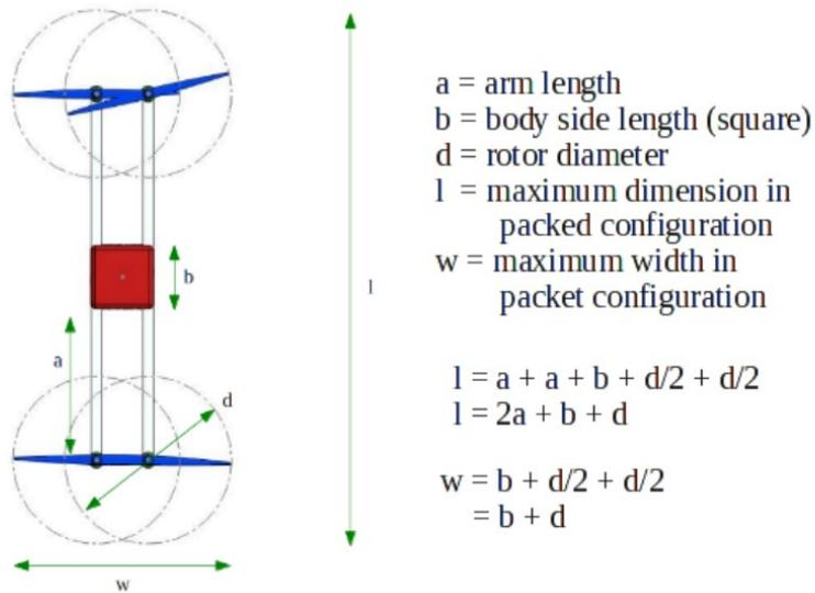
**Figure 10: Quadrotor dimensions in packed configuration.**
