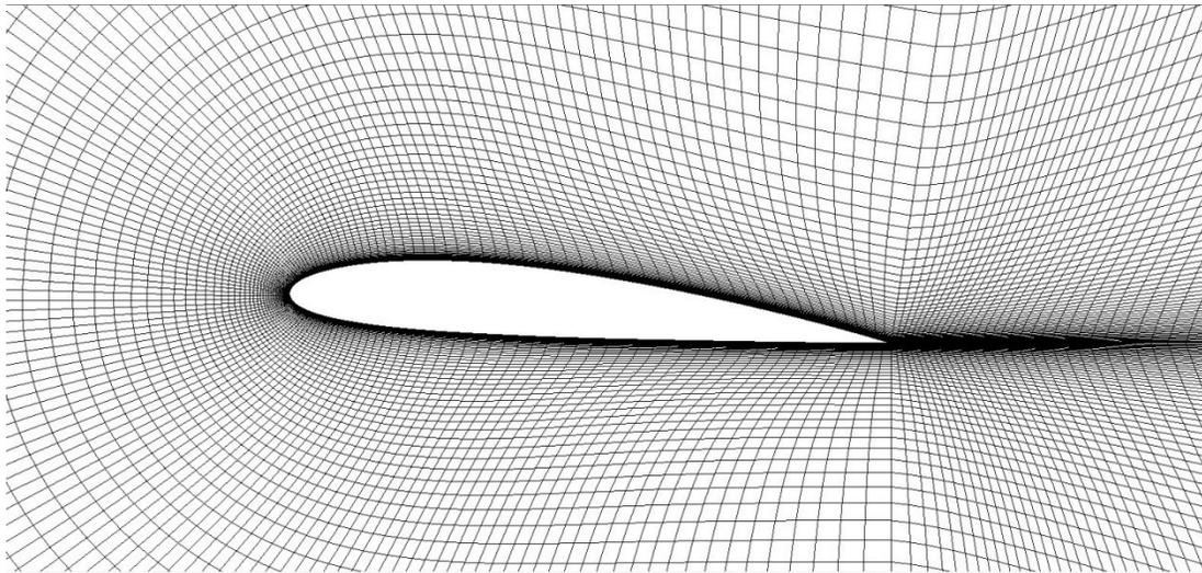
**Figure 36: Structured grid around NACA 2412 section.**
