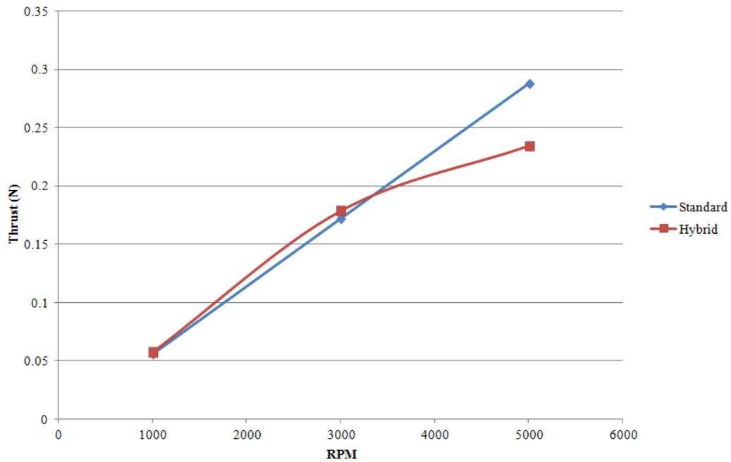
Figure 45: Thrust vs. RPM for standard and hybrid rotors.
