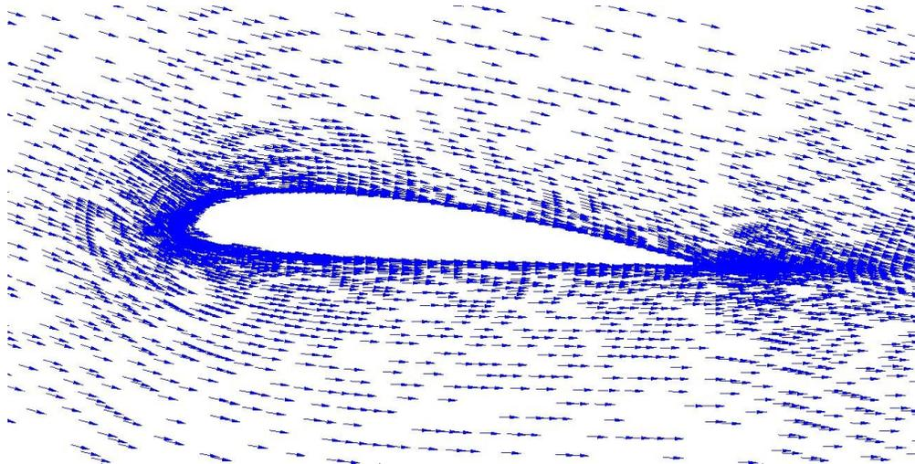
Figure 43: Velocity vectors around NACA 2412 section.
