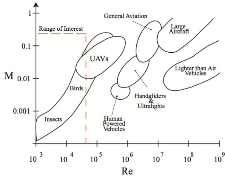
Figure 17: Reynolds number ranges for various flight vehicles. [7]
