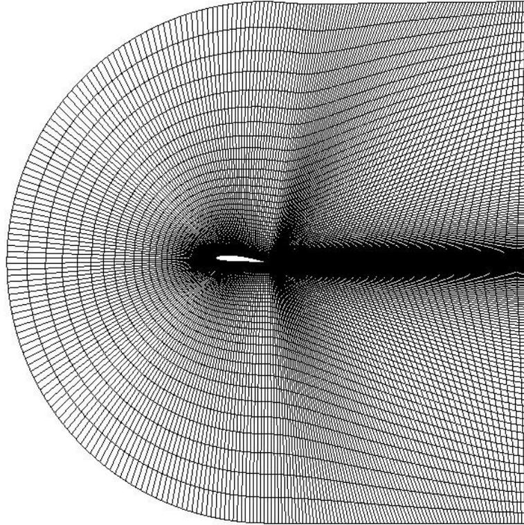
**Figure 35: Structured grid around standard rotor.**
