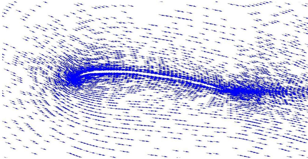
**Figure 44: Velocity vectors around Goe 417a section.**
