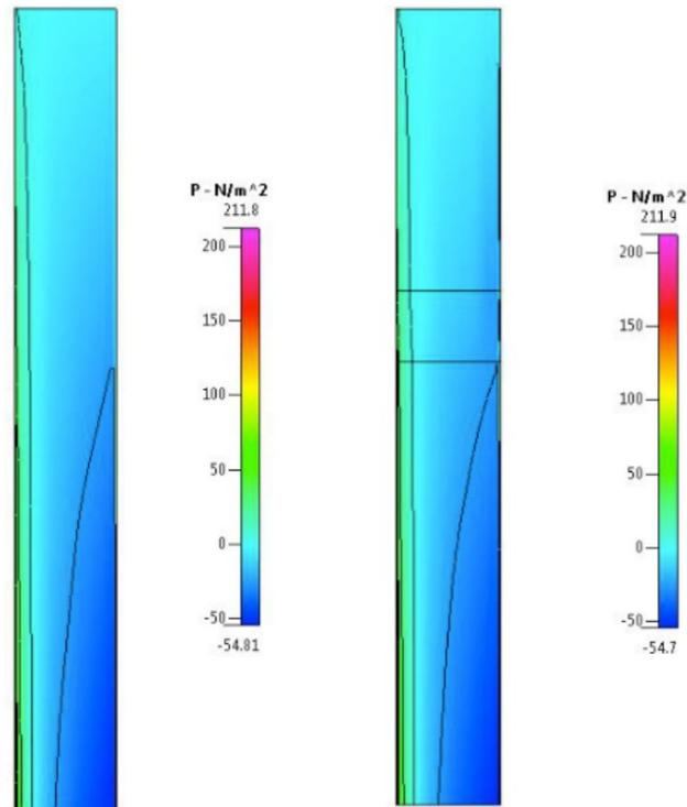
Figure 41: Pressure contours on upper surfaces of standard (left) and hybrid (right) rotors at 3000 RPM.
