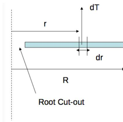
Figure 29: Elemental rotor sections. [8]
