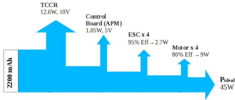
Figure 14: Power distribution for platform and components.
