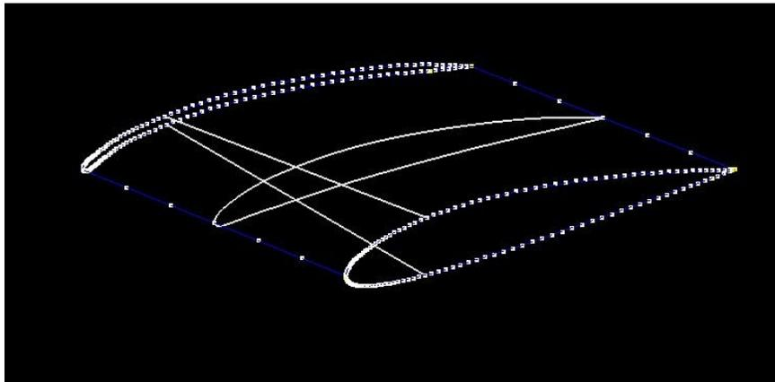
**Figure 38: Interpolated grid section between NACA 2412 and Go 417a.**
