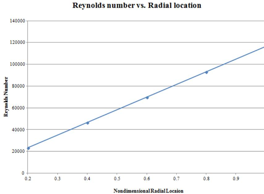
**Figure 47: Reynolds number as a function of radial location for the 16.8" at 3000 RPM.**
