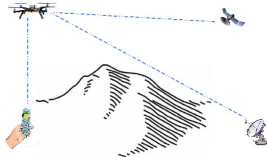
**Figure 3: Aerial relay platform enabling LOS to receiver and/or satellite, solving the obstruction problem as shown in Figure 1.**
