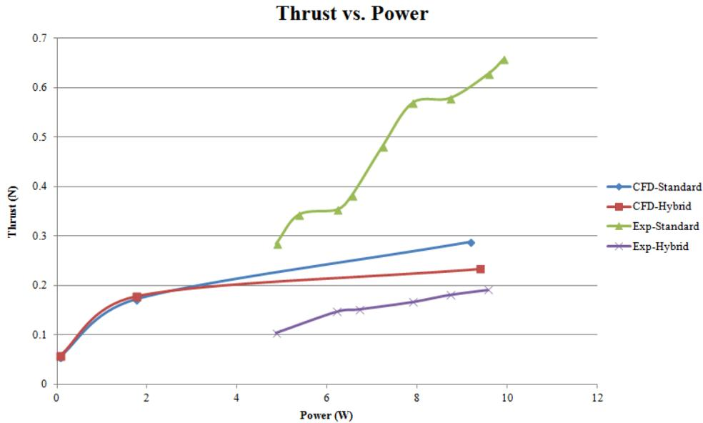
Figure 52: Thrust vs. power required plot comparing CFD and experimental results.
