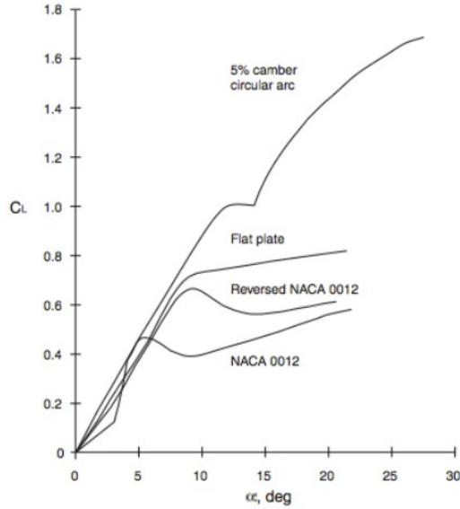
Figure 26b: Coefficient of lift vs. angle of attack for NACA 0012, flat plate, and cambered plate. [7]
