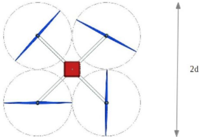
**Figure 11: Maximum diameter rotors. The rotor disk [diameter] is marked by the gray hatched circles.**
