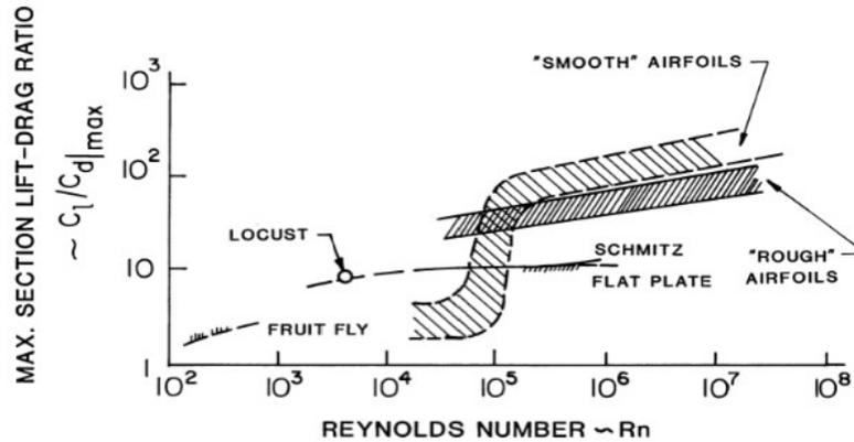
Figure 28:  $C_l/C_d_{max}$  for various flight bodies over increasing Reynolds numbers.
