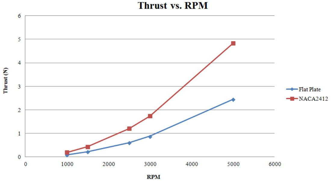
Figure 32: Thrust vs. RPM for flat plate and NACA 2412 from BEM.
