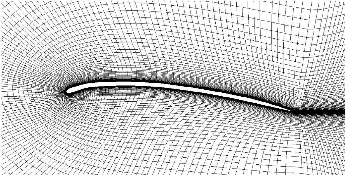
**Figure 37: Structured grid around Goe 417a section.**
