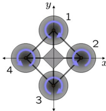
**Figure 7: : Fundamental control of a quadrotor. With each rotor rotating in these specified directions, the net yaw torque on the vehicle is null. [15]**
