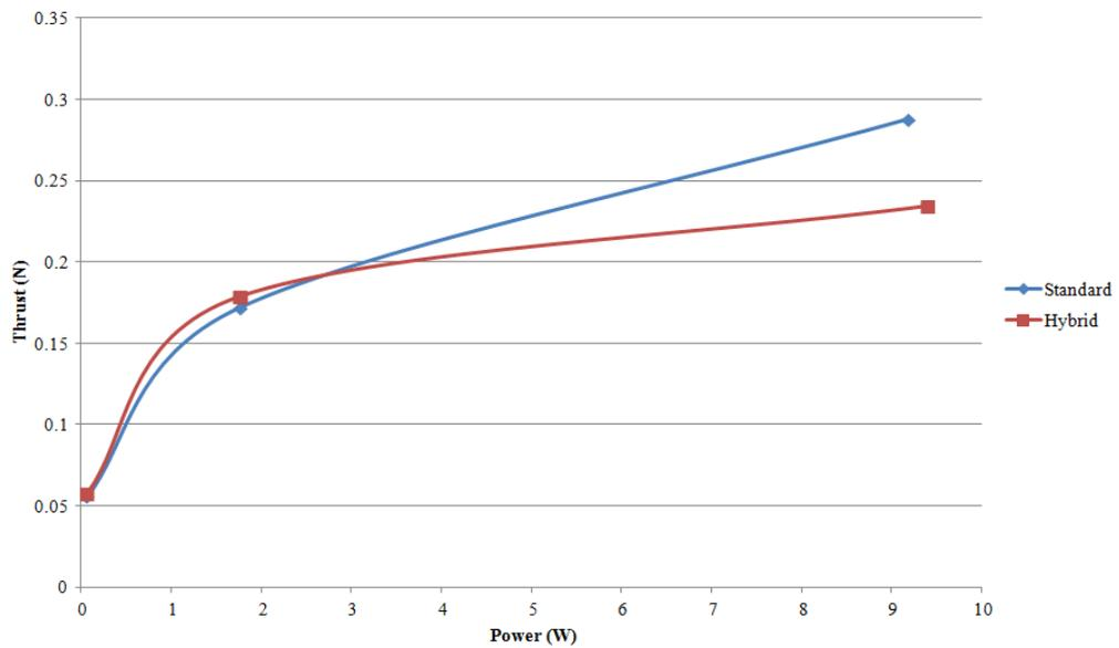
Figure 46: Predicted thrust vs. power for standard and hybrid rotors.
