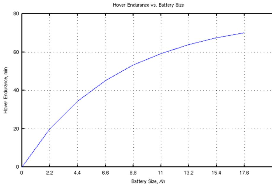
Figure 15: Hover endurance vs. battery capacity. Each tick along the abscissa is one 2200mAh battery.
