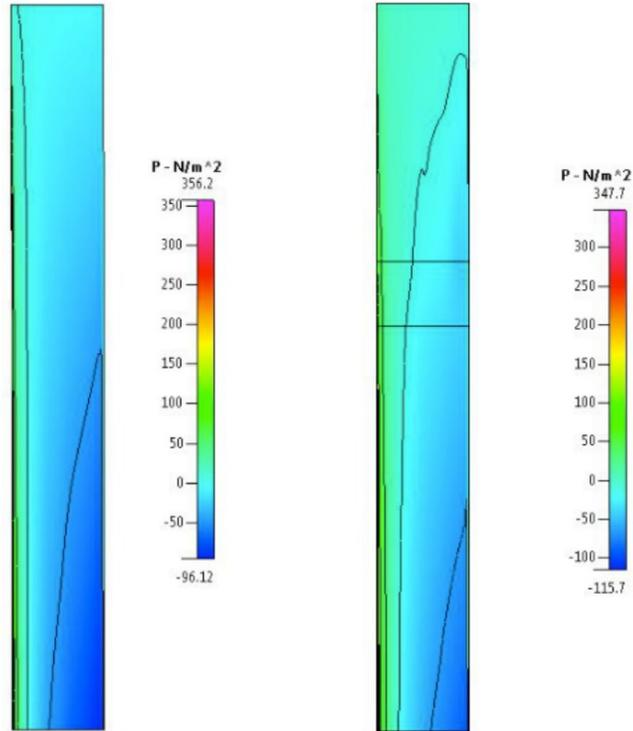
Figure 42: Pressure contours on upper surfaces of standard (left) and hybrid (right) rotors at 5000 RPM.
