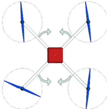
**Figure 9: Quadrotor prior to folding in flight-ready configuration. Arms rotate inwards 45 degrees.**
