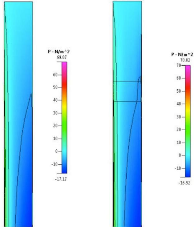
Figure 40: Pressure contours on upper surfaces of standard (left) and hybrid (right) rotors at 1000 RPM.
