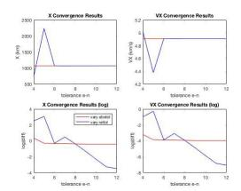
Fig. 43 Vary Tolerance: LEO, ODE45, 600hour, J2+Lunar (Convergence Results)
