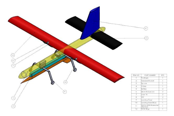
Figure 14: Preliminary layout of the Airplane
