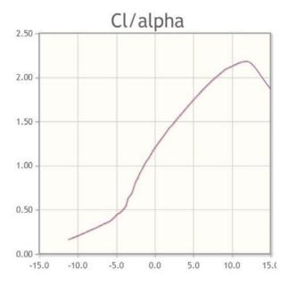
Figure 2: Coefficient of Lift vs. Angle of Attack
