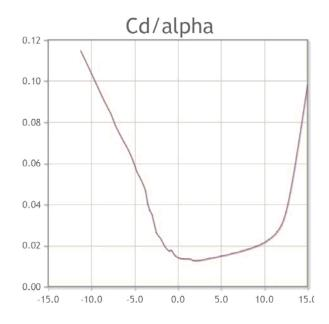
Figure 3: Coefficient of Drag vs. Angle of Attack
